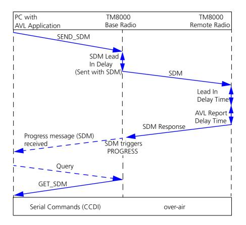
This sequence of events can be simplified by choosing the programming option "output SDMs automatically" for the base radio (available in TM8000 release 3 programming software).
